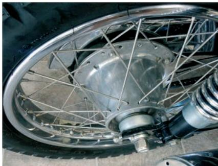
Conical rear hub on a T150V.
