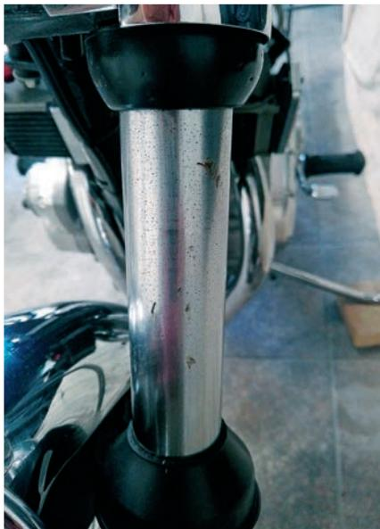
Check fork stanchions for signs of pitting, which can cause oil leaks.
